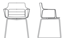
Poltrona monoscocca, telaio in tubo cromato Mono-shell chair; chrome plated frame L 61/43 P 50/40 HT 80 HS 44
