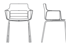
Poltrona monoscocca, base 4 gambe Mono-shell chair, 4 legs base L 61/43 P 50/40 HT 80 HS 44
